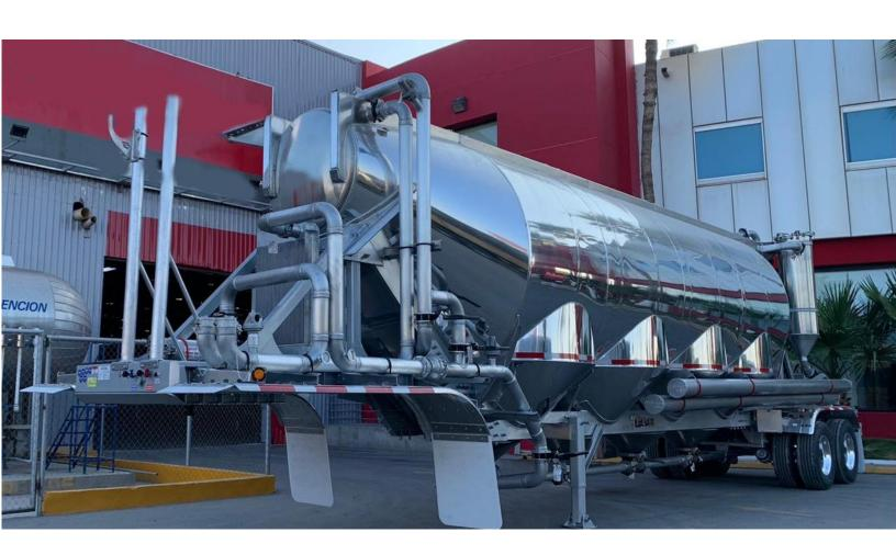
Four Hopper – 1636 Cu. FT Capacity
